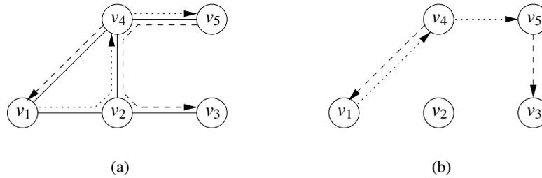
Figure 1.3: (a) Lightpaths in an optical network; (b) The virtual topology that results from the established lightpaths.
