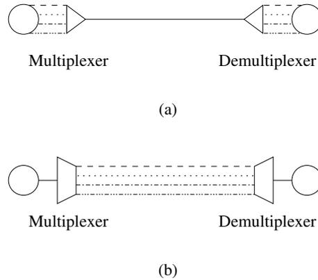
Figure 1.1: A WDM system with four wavelengths. (a) Technical view; (b) Presentation of the channels on the fiber.
