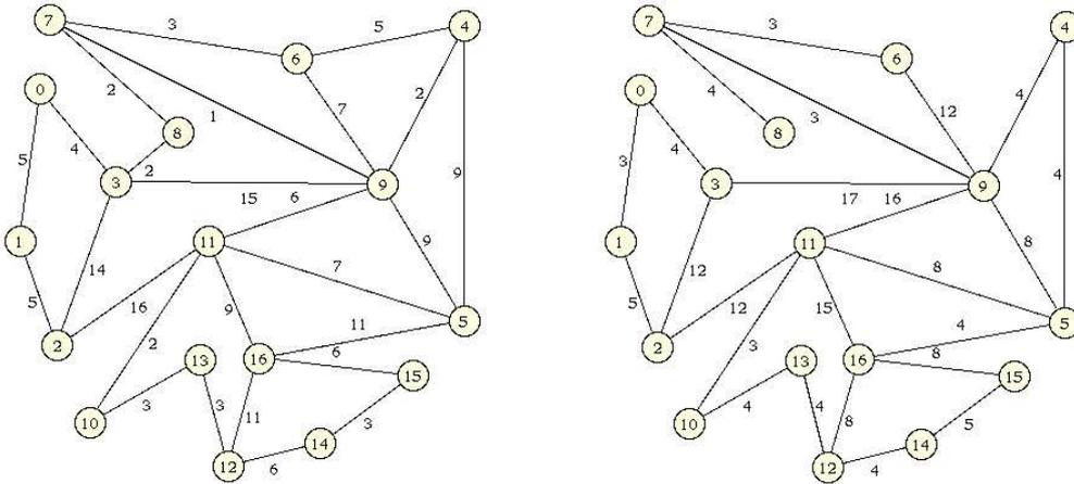
Figure 5.1: The 17-nodes network with shortest path (left) and with low cost dimensioning (right).
