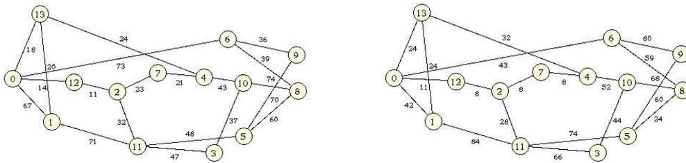
Figure 5.2: The 14-nodes network with shortest path (left) and with low cost dimensioning (right).
