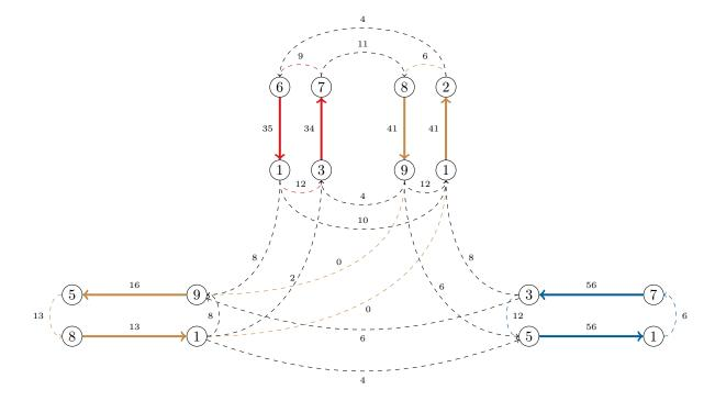
The network  $\mathcal{E}$  is equipped with a periodic timetable  $\pi : V(\mathcal{E}) \to \{0, 1, \dots, 9\}$  with period time T = 10. Each vertex v is labeled with  $\pi(v)$ . Moreover, each edge carries a length compatible with  $\pi$ . The solid arcs represent driving activities, whereas the dashed arcs mark turnaround activities.
