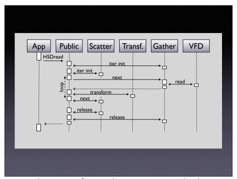
[cont.] This is a high level sequence diagram of a read operation inside the HDF5 Library. It's basically built up of two iterators. One is gathering data from a file, the second one is writing the data to the application's memory. Only the read operations are of interest for understanding the remote performance. [NEXT SLIDE]
