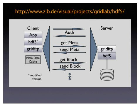
**[cont.]** We chose to use gridftp which is an extension to the standard FTP protocol. It provides server side processing information. The overall architecture of the remote access looks like this. All our modifications to existing software are available at the url at the top.
