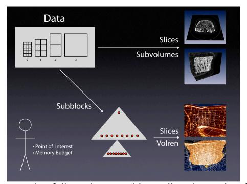
[cont.] The volumetric data is stored at full resolution. Additionally, a hierarchy of lower resolution preview versions is generated. To preserve thin structures in our data we use a maximum filter in the first downsampling step. Further levels are generated by averaging the voxel values of the level just below. [PRESS] Accessing subvolumes of a specific resolution is used for simple slicing or for retrieving subvolumes to be stored locally or be visualized using various techniques.
