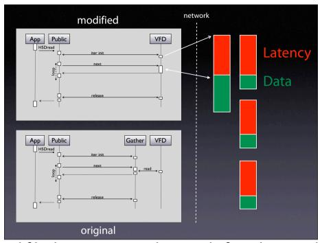
**[cont.]** We changed how a virtual file driver is accessed. Instead of sending unrelated read requests it is given the opportunity to see the whole selection. During iterator initialization it sends this request to the remote side. Processing there starts right away. Data is sent back and delivered to the HDF5 library on demand.
