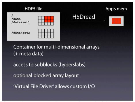
[cont.] It provides a container for multidimensional arrays. Several of these arrays can be stored together with accompanying meta data. They can be organized in a file system like structure.
