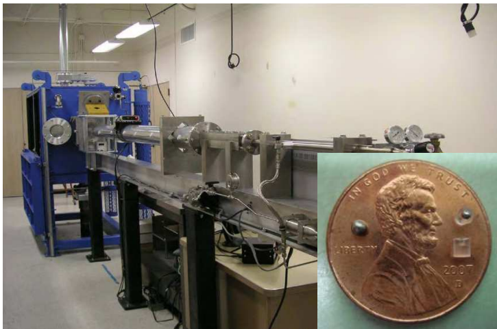
Figure: Caltech's Small Particle Hypervelocity Impact Range (SPHIR) : a two-stage light gas gun that launches 1–50 mg projectiles at speeds of 2–10 km · s -1 .
