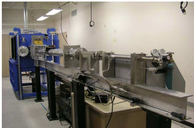
Figure: Caltech's Small Particle Hypervelocity Impact Range (SPHIR) : a two-stage light gas gun that launches 1–50 mg projectiles at speeds of 2\text{--}10\text{ km} \cdot \text{s}^{-1} .
