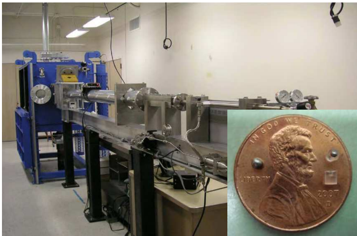
Figure : Caltech's Small Particle Hypervelocity Impact Range (SPHIR) : a two-stage light gas gun that launches 1–50 mg projectiles at speeds of 2\text{--}10 \text{ km} \cdot \text{s}^{-1} .
