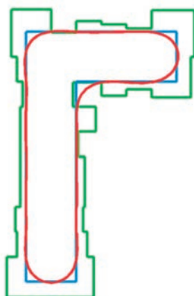
Figure 7: An example of Optical Proximity Correction . The green mask produces the red structure after photolithographic imaging (illustration from Wikipedia).
