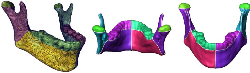
Fig. 3: Patch decomposition of mandibular bone for the construction of the statistical shape model.
