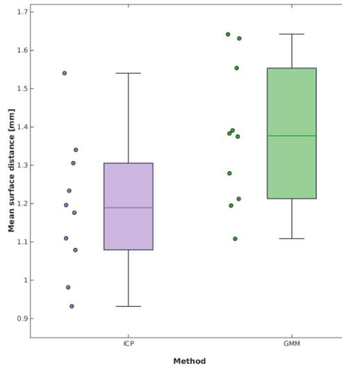
Fig. 4: Mean surface distance between the SSM fit to the point clouds and the ground truth surfaces. The plot showing mean value ± std. deviation with Whisker bars at min and max value.
