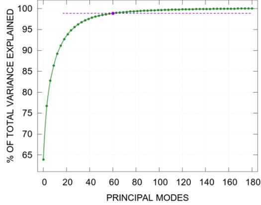
Fig. 2: Percentage of total variance explained with respect to the number of shape modes for the used SSM consisting of 184 training shapes.
