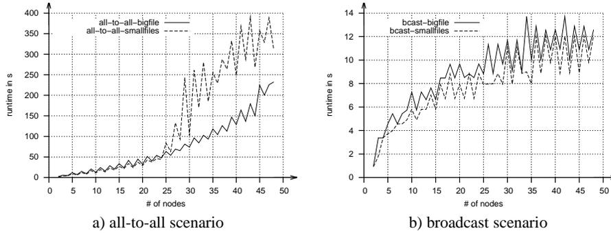
**Fig. 4.** *nsync* performance on a PC cluster.
