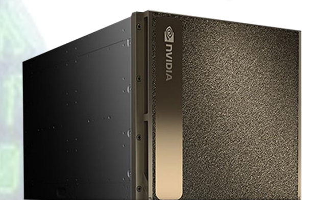
NVIDIA DGX-2 Deep Learning System 16x NVIDIA V100 GPU, 512 GB GPU Memory
