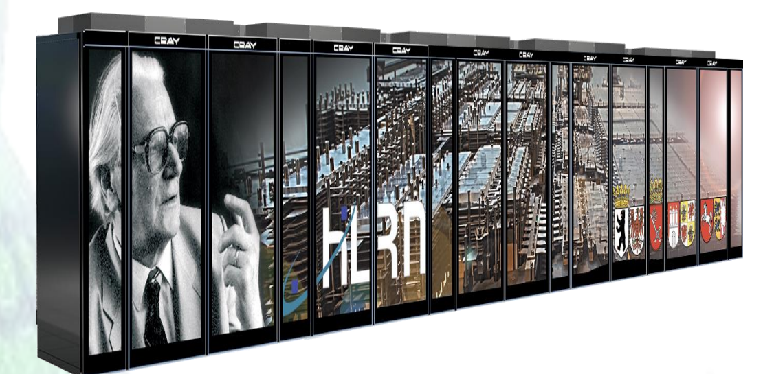
ZIB/HLRN HPC: 1872 nodes, each equipped with 2 Intel CPUs consisting of 12 cores. 120 TB of main memory
