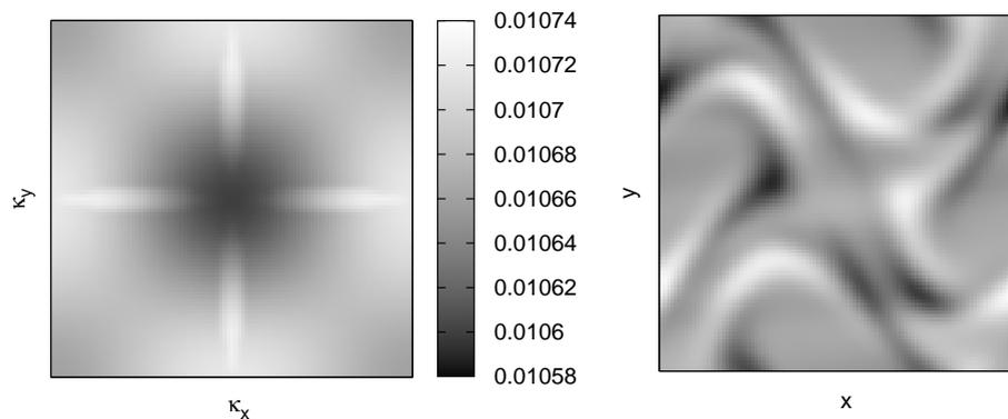
Figure 5: Largest Lyapunov exponent as a function of  $\kappa_x, \kappa_y$  (left) and a corresponding pattern at a point of its maximum (right) evaluated at  $a = 3.1, c = -4.1, U = 3.5$ . Maxima of LE correspond to  $\kappa_x = 0, \kappa_y = \pm 0.4$  and  $\kappa_x = \pm 0.4, \kappa_y = 0$ .
