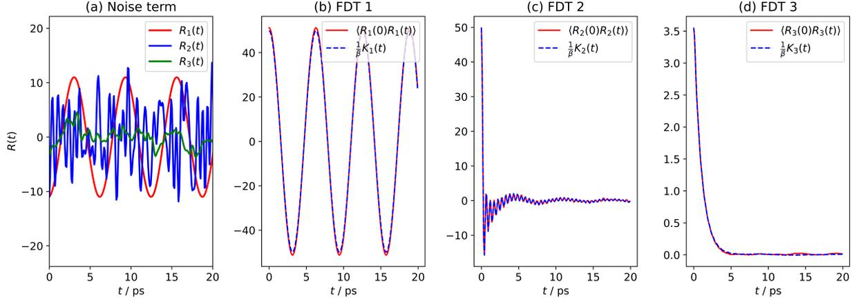
FIG. 1. Noise term (a) and FDT (b,c,d) for three different set of parameters  $\omega_i, k_i, m_i$  with  $N = 2000$  oscillators in thermal equilibrium.
