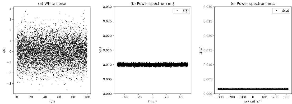
FIG. 5. Example of white noise (a) and power spectrum (b,c) with ordinary and angular frequencies.
