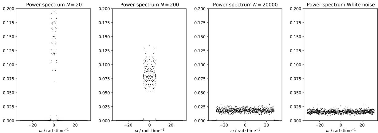
FIG. 3. Power spectrum of the noise term with  $N = 20, 200, 20000$  oscillators in thermal equilibrium (a,b,c) and power spectrum of the white noise (d).
