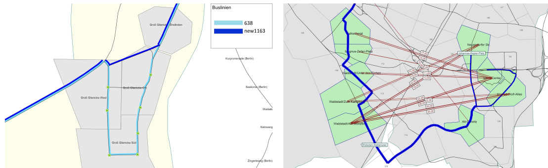
Figure 9.4: Left: Comparing the routes of the line 638 in the P10 plan and the line new1163 in the OPT plan. Right: OD pairs with a direct (i. e., transfer free) connection provided by the bus lines new28256 and new30369. The numbers on the red lines correspond to the demand of the associated OD pair; graphics generated with VISUM [83].
