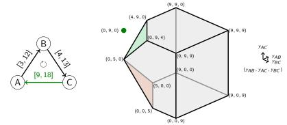
Flip AC: In the flipped PESP instance w.r.t.  $F = \{AC\}$ , the change-cycle inequality is  $6\overline{y}_{AB} + 6\overline{y}_{BC} + 6\overline{y}_{CA} \ge 24$ , which in the original instance translates to the flip inequality  $6y_{AB} + 6y_{BC} + 6(9 - y_{AC}) \ge 24$ . Simplifying, we obtain
