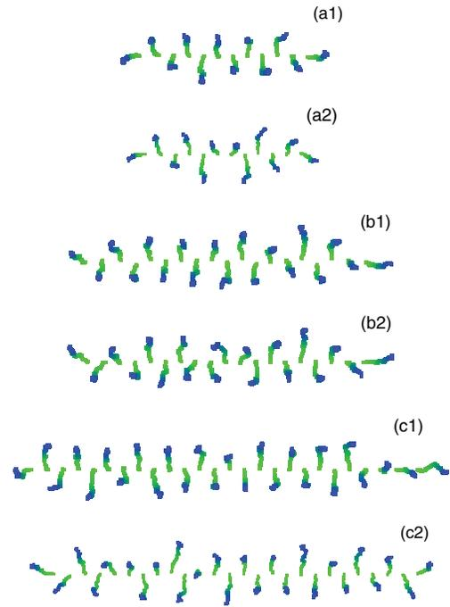
FIG. 8. Particle trajectories showing nonequilibrium expansion patterns for chains with different number of colloids:  $N = 12$  (a),  $N = 19$  (b), and  $N = 26$  (c) obtained for  $b = 0.8b_c$  and  $\alpha = 30$ . Panels (a1), (b1), and (c1) demonstrate zigzag patterns without defects, while panels (a2), (b2), and (c2) show patterns with simple imperfections.
