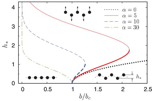
FIG. 2. Bifurcation diagram showing equilibrium states for different values of  $\alpha$ . The line state  $h_* = 0$  exists for all  $\alpha$  and is stable for  $b < b_c$ . The solution describing the stable equilibrium zigzag state ( $db/dh_* > 0$ ) is shown by bold lines; it exists for traps with  $\alpha < \alpha_c$  in the range of  $b_c < b < b_{**}$  with  $b_{**}$  the turning point, see Eq. (25). The branches where  $db/dh_* < 0$  (lines of normal thickness) are unstable.
