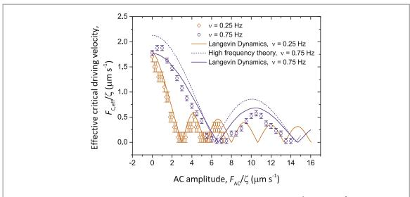
**Figure 7.** Critical driving velocity,  $F_{\text{C,eff}}/\zeta$ , as a function of modulation amplitude,  $F_{\text{AC}}/\zeta$ , for  $\nu=\frac{1}{4}$  Hz and  $\nu=\frac{3}{4}$  Hz. Symbols show experimental data, solid lines show LD simulation results, and the dashed line shows the high frequency approximation.
