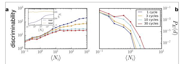
**Figure 11.** Discriminability and associated probability of a reading error as a function of the average particle number for various numbers of read—reset-cycles. The inset denotes the optimal reading and reset voltages, i.e., those for which the reading resistance drops to a minimum and the reset resistance is close to the value reached in the writing cycle, respectively. Other parameters as in figure 2.
