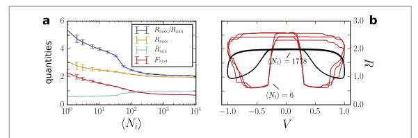
**Figure 5.** Effects due to enhanced stochasticity caused by different mean number of particles per lattice site  $\langle N_i \rangle$ . (a) Resistance minima and maxima, and hysteresis loops in the R-V diagram as in figure 3, albeit as a function of  $\langle N_i \rangle$ . (b) Sample R-V plots for various  $\langle N_i \rangle$ . All parameters as in figure 2.
