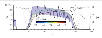
**Figure 4.** RS dynamics with enhanced fluctuations due to decreased average vacancy number at constant  $\langle N_i \rangle / N_0 = 0.01$ . Colored faces are the standard deviation around the mean value, inside which one sample distribution for each  $\langle N_i \rangle$  is shown. Curves given at different time points of the driving cycle, as indicated by the color scheme.
