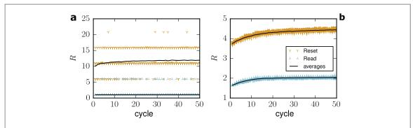
**Figure 10.** Resistances after several repeats (=cycles) of read and reset operations, for different average particle numbers per lattice site, (a)  $\langle N_i \rangle = 0.2$  and (b)  $\langle N_i \rangle = 178$ . Other parameters as in figure 2.
