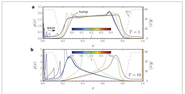
**Figure 6.** Vacancy distribution of RS modeled by numerical integration of the corresponding Burgers equation (16). Various time points of the switching cycle indicated by the color coding. Parameters as in figure 2, for driving periods (a) T=1 and (b) T=10.
