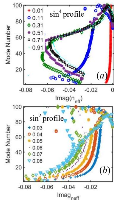
Imaginary part of the effective indices of various modes for (a) a ‘good’ and (b) a ‘poor’ absorption profiles in the ABC. Various curves correspond to different strength of the absorption as shown. Layer width is 24% of the total window.
