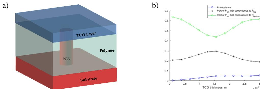
Fig.1. (a) Schematic of the modeled system containing the TCO layer as a top contact. (b) Absorptance in the TCO and far-field emission to the top and bottom sides as a function of TCO thickness.
