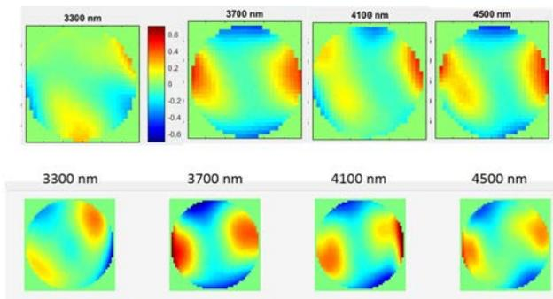
Fig.2: Simulated (bot.) vs. measured (top) wave-fronts
