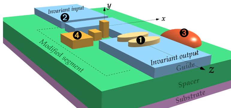
Fig. 1.: Typical waveguide and possible obstacles. Any bounded modification of the permittivity of the invariant structure can be considered: Ellipsoidal patches above the guiding layer ①, holes ② in the guiding layer, obstacles or resonators next to the waveguide ③ or even a combination of all ④...
