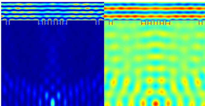
*Inverted plasmonic lens (grey structure indicating the metallic coating), illuminated by a plane wave from above. Intensity (left) and amplitude distribution (right). In the desired distance the lens produces a focal spot.*
