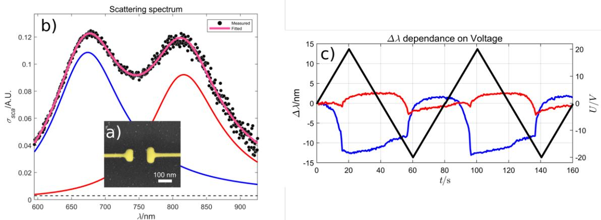
Fig. 1. First results of the device: a) SEM image of the geometry; b) white light scattering (black dots) and fit of the two resonances (blue and red curves) of the structure in a) without applied voltage; c) Applied voltage (black curve) and corresponding measured changes  $\Delta\lambda$  in both antennas resonances in ambient conditions. Not depicted are the vanishing curves for the same measurement when performed in a  $N_2$  atmosphere.
