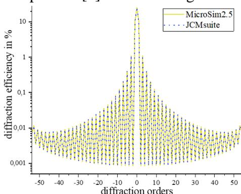
*Comparison of the diffraction efficiencies of MicroSim2.5 and JCMSuite*
