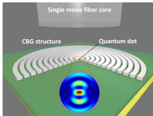
Fig. 1. Illustration of a hybrid CBG with an embedded QD, aligned to an optical single-mode fiber.
