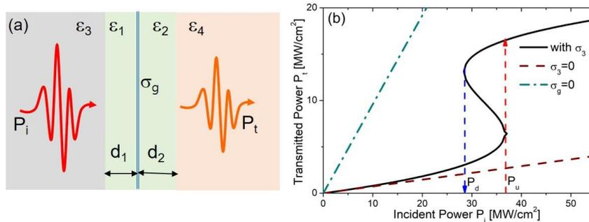
*Figure (a) System configuration: graphene embedded in four dielectric layers. (b) THz OB of graphene at the interface between two dielectrics  $\epsilon_1=\epsilon_3=2.25$  and  $\epsilon_2=\epsilon_4=1$  can be obtained at 1 THz with a high Fermi-energy of graphene  $E_f=1.2\text{eV}$  and is bounded by two limits ( $\sigma_g=0$  for no graphene and  $\sigma_3=0$  for zero optical nonlinearity)*
