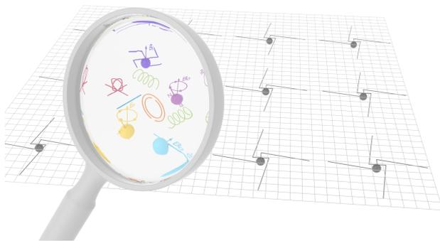
*Conceptual illustration of the modular analysis. An arbitrary scatterer (located in a two-dimensional array of equivalent scatterers in this example) with a complex polarization response is decomposed into a combination of responses from several basic modules with known basic electromagnetic properties.*
