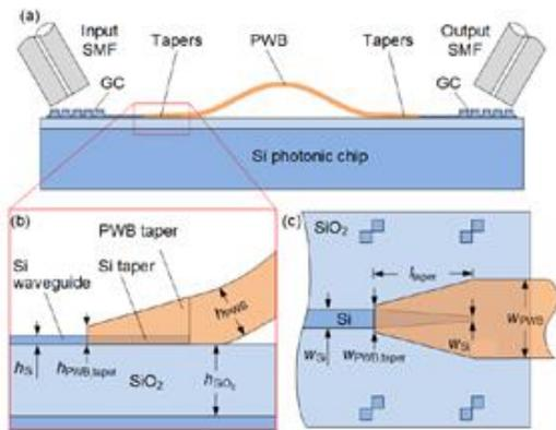
*Schematic and field profile of the adiabatic waveguide coupler.*
