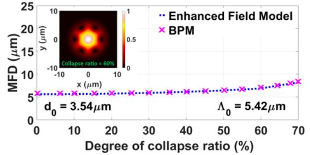
Fig. 1. MFD against collapse ratio at  $1.55\mu\text{m}$ .
