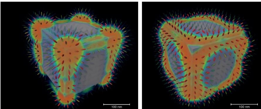
*Tomographic reconstruction of photonic LDOS for corner (left) and edge (right) modes of a single MgO nanocube. The scale bar is 100 nm.*
