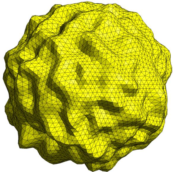
Fig. 1. Unstructured mesh of a rough sphere with radius  $r$ , rms roughness  $R_q = 0.05$ , correlation length  $l/r = 0.15$  and element size  $h/r = 0.05$ .
