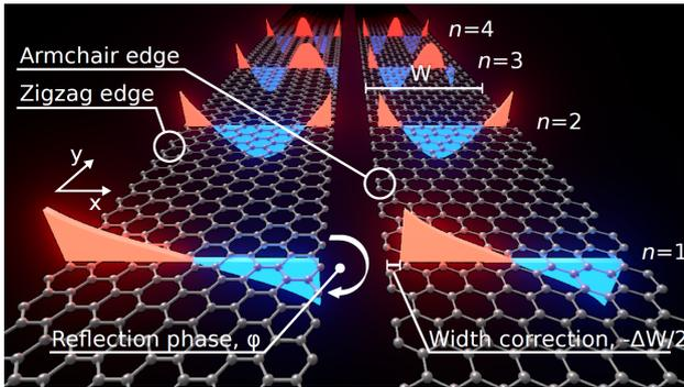
Induced charges for dipolar and higher-order plasmons on zig-zag and armchair graphene nanoribbons. Red and blue correspond to negative and positive charges. Figure from Ref. [6].
