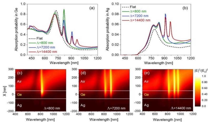
Absorption probability in (a) Ag, and (b) Ge layers for different periods. The dash lines show the absorption of flat structures. (c) Normalized electric field intensity corresponding to gratings with  $\Lambda=800$  nm, (d)  $\Lambda=7200$  nm, and (e)  $\Lambda=14400$  nm within their layer configuration.
