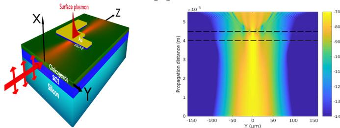
Fig. 1. Left: Scheme of one modeled structure with beam injection and axis definitions, the nonlinear layer is the dark green one. Right: Color map in log scale of the beam intensity evolution along the  $Y$ -axis versus propagation inside the full structure for TM polarization with a  $500 \mu\text{m}$  wide gold stripe in the nonlinear regime. The dashed lines represent the limits of the gold stripe.
