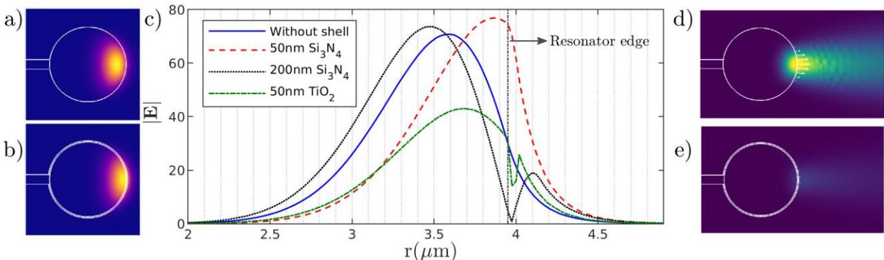
Electric field profile of the 93<sup>rd</sup> azimuthal mode in a micro-toroid a) without and, b) with a 50 nm  $\text{Si}_3\text{N}_4$  shell, and c) the electric field intensity on the equator for various shell thicknesses and compositions in comparison with the toroid without any shell. The radiation energy flux from a micro-toroid a) without and, b) with a 50 nm  $\text{Si}_3\text{N}_4$  shell.
