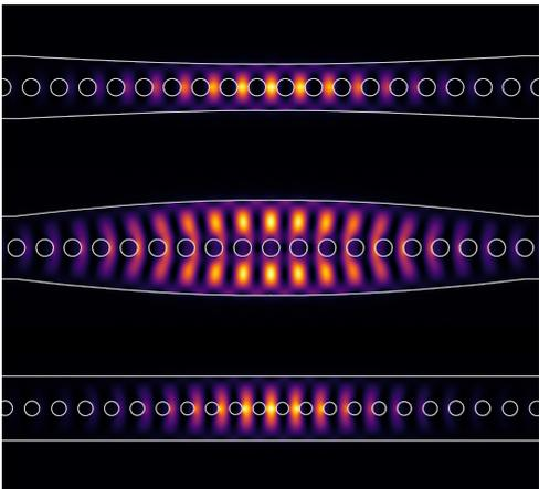
**Figure:** Dielectric structure and total electric field density of the three optimised cavity designs. Top and center: quadratic tapering of waveguide width (Deterministic design approach). Bottom: linear tapering of hole radii and distances, additional defect length (Mode-matching design approach).
