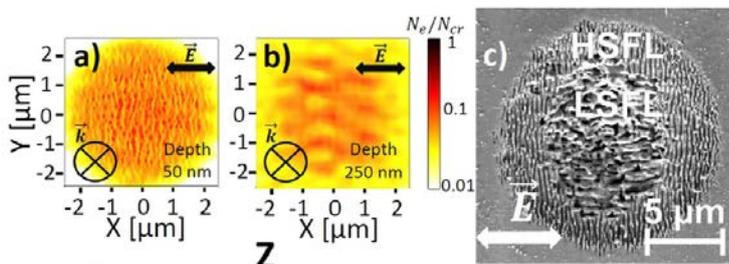
(a, b) Normalized laser-induced electron density distributions in silica calculated by 3D-FDTD for a 120 fs laser pulse (800 nm) at two different depths from the rough surface. (c) SEM micrograph of LIPSS on a quartz surface after irradiation with 20 laser pulses (150 fs, 800 nm, 5.8 J/cm<sup>2</sup>) [3].
