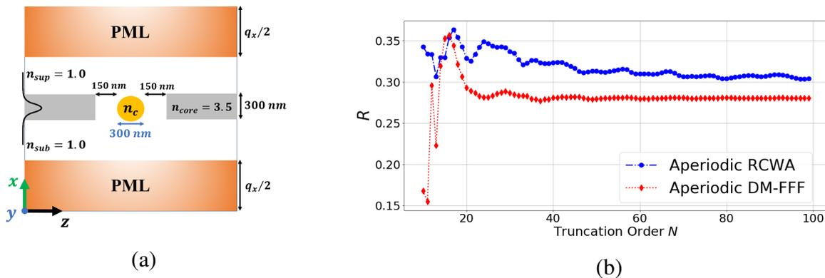
Fig. 1.: (a) Integrated optic structure with  $n_c = 1.0 + j4.0$ . PMLs of thickness  $q_x$  are surrounding the structure b) Evolution of the reflection coefficient  $R$  w.r.t  $N$  using the a-RCWA and a-DM-FFF
