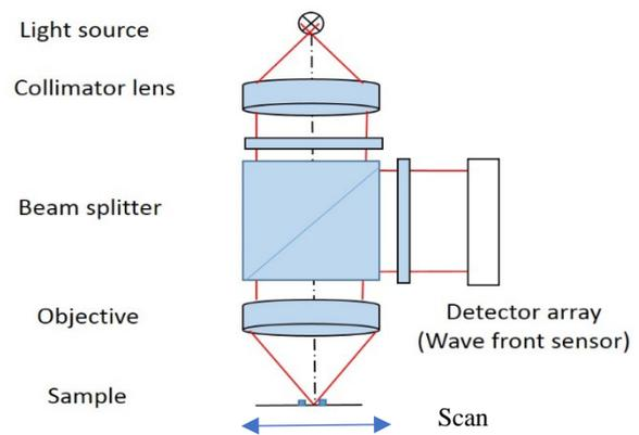
Figure 1: Basic principle of SCFT
