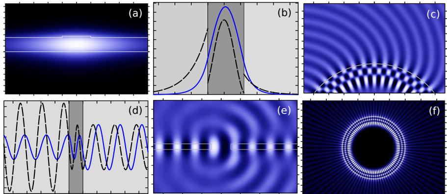
(f) Whispering-gallery resonance of a circular dielectric rod, interference of clockwise and anticlockwise propagating WGMs of second radial order, field modulus.
