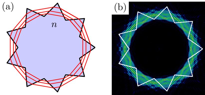
Figure 1: (a) The ray dynamics in the microstar cavity with nine spikes and adjusted refractive index  $n$ . In (b) the intensity mode pattern of a long-lived optical mode is shown.
