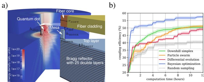
**a)** Visualization of the light field intensity of a fiber-coupled single-photon source, which is optimized w.r.t. the depicted parameters (black). **b)** Average of the best seen coupling efficiency for different optimization approaches versus the total computation time.
