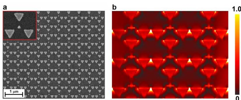
Fig.1: SEM image (a) and simulation of near-field distributions (b) of the octupolar nanopattern.
