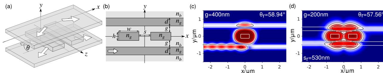
Fig. 1. Oblique excitation of a micro-cavity: 3-D sketch (a), cross section view (b) and field plots of  $|E|$  at resonance for one (c) or two (d) cavities with waveguide parameters  $n_g = 3.45$ ,  $n_b = 1.45$ ,  $d = h = 0.22\mu m$ ,  $w = 0.5\mu m$ , variable gap  $g$  and separation  $s$ .
