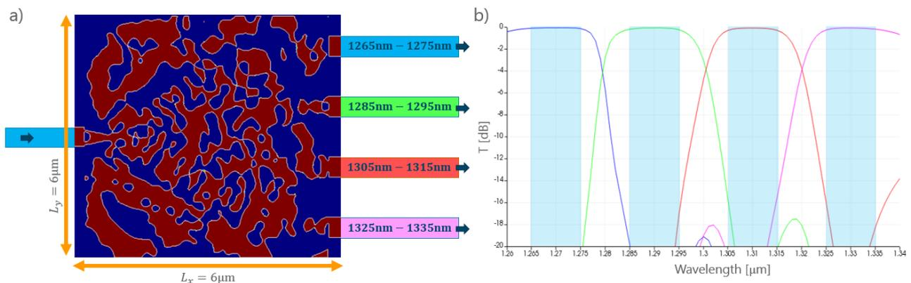
Fig. 1: (a) Result of a topology optimization of a 4-channel CWDM demultiplexer. (b) Corresponding transmission spectra of the four channels.
