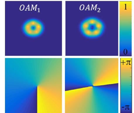
Fig. 2 Amplitude (top) and phase (below) of the generated OAM modes.
