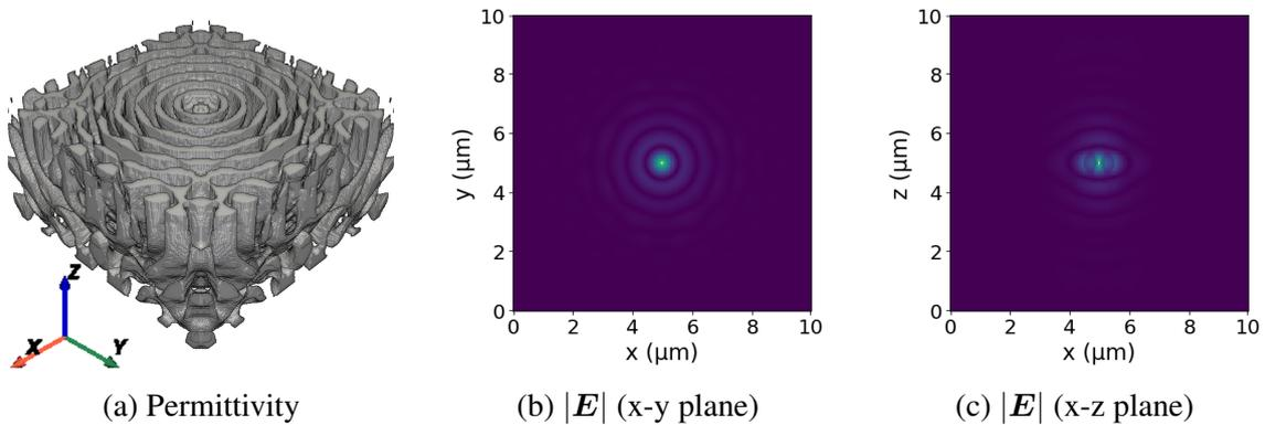
Fig. 1.: A 3D topology-optimized optical cavity with a resonance wavelength of  $1.5 \mu\text{m}$  and a refractive index contrast of  $\Delta n = 0.6$ . The designable area consists of a cube with a volume of  $10 \mu\text{m}^3$ . Shown is (a) a cross section of the permittivity distribution centered in the x-y plane as well as the absolute electric field at the cavity center in the (b) x-y and the (c) x-z plane.
