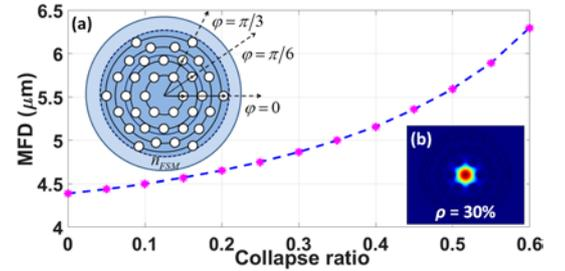
Fig.1. MFD against collapse ratio.
