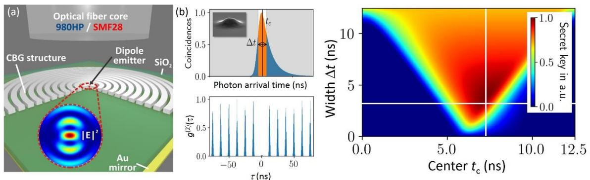
Fig. 1. (a) Illustration of a telecom-wavelength quantum light source based on a hybrid circular Bragg grating device coupled to an optical single mode fiber [2]. (b) Performance optimization of single-photon QKD exploiting 2D temporal filtering using a receiver module developed for polarization encoding [3].
