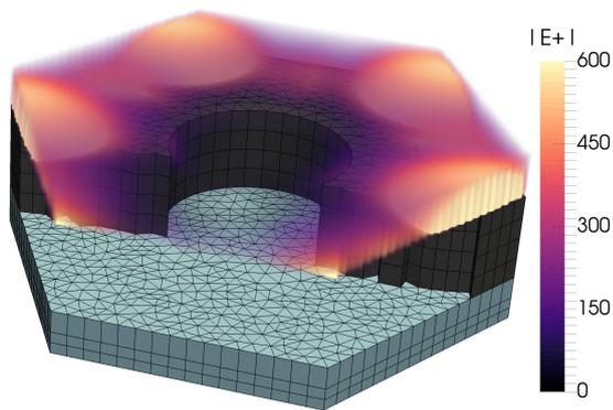
*The enhanced intensity of light in the near field of a photonic crystal slab due to the presence of a leaky mode. Part of the FEM mesh used for simulation of the unit cell is also shown.*
