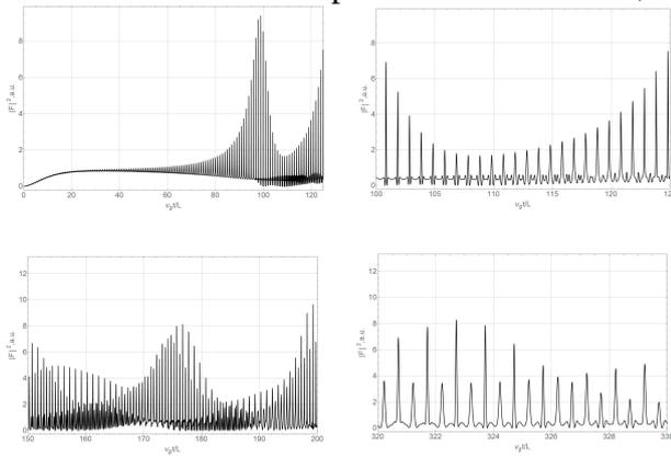
*Examples of the modelling results. The top row displays the dynamics of the pulse propagation as a whole, unidirectional case with the dispersion. The bottom row displays the close up cuts of the regimes where the fibre has received non-reciprocal phase shift because of the slight rotation introduced, and there is a highly reflective intra-cavity mirror installed. Introducing of the Rayleigh scattering significantly changes the dynamics.*
