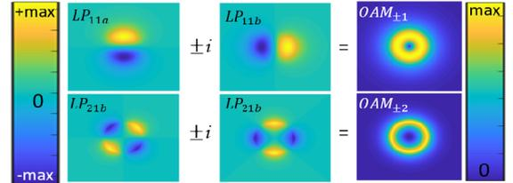
Fig. 1 Scheme for generation of OAM modes using pairs of LP modes.
