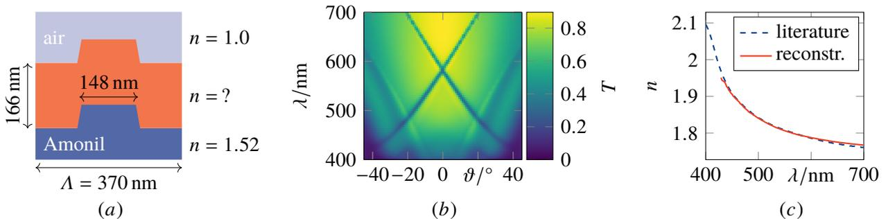
**Figure.** Numeric validation of proposed method. (a) Material under test (red) on photoresist (Amonil) nanostructure. (b) FDTD-simulated angle-resolved transmission spectrum for OLED material NPB. (c) Refractive index of NPB reconstructed from the guided-mode resonance positions in (b) and the Bragg equation, compared to the literature value used in the simulation.
