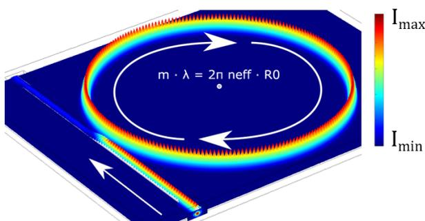
*Intensity distribution in a silicon microring resonator with bus waveguide at resonance.*
