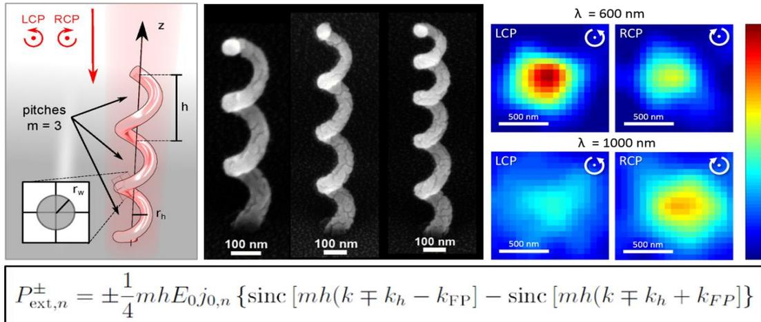
**Figure** From left to right: Geometrical setting, scanning electron micrographs of silver coated helices, extinction maps of a helix with 4 turns. The analytical formula quantifies the excitation efficiencies for all types of resonances.
