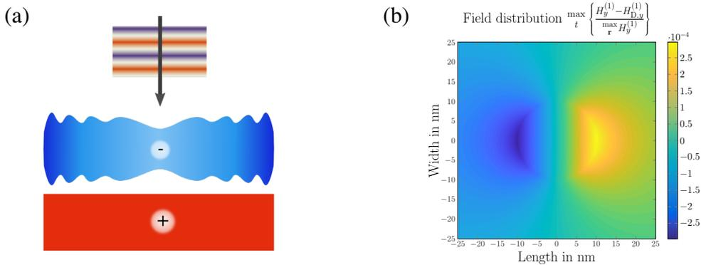
(a) Sketch of a plane wave excitation of a hydrodynamic metal. (b) Influence of the drift current on a spherical silver scatterer: The response of a silver scatterer is computed numerically for the linearized hydrodynamic material with and without additional drift-current. The difference between these calculations is displayed on the right figure.
